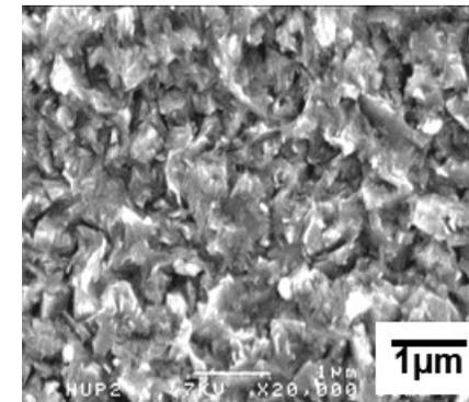
Crystallization due to prolonged stages at  $T > T_g$
