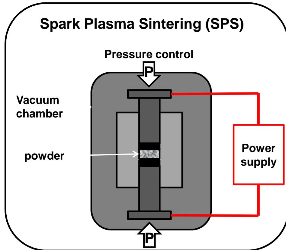
Faster temperature ramps reached with SPS
