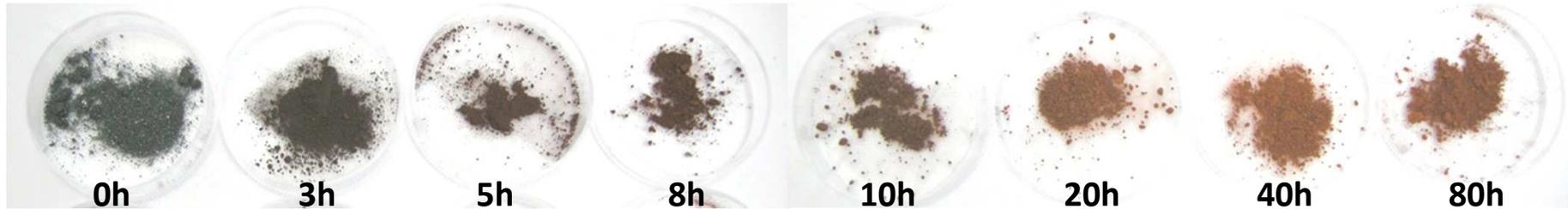
Progressive reaction between the elements and lowering of particle size
