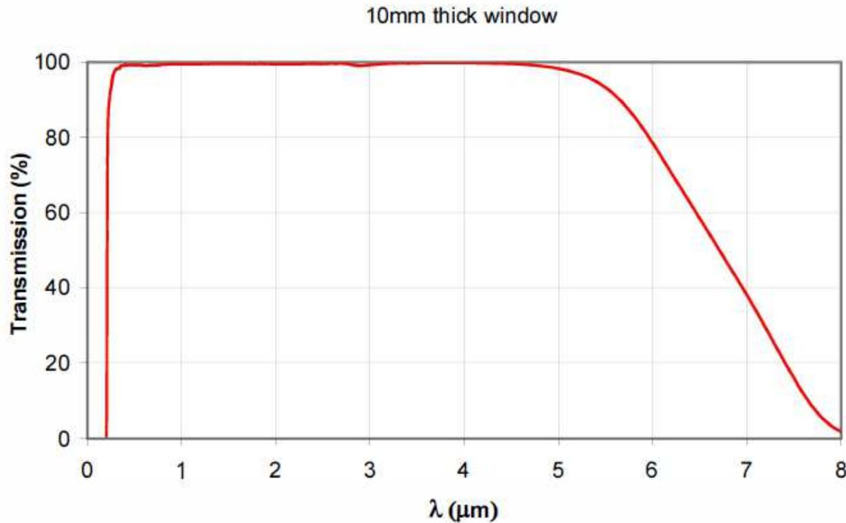
Figure 1: transmission window of Fluorozirconate glass sample (10 mm tick)
